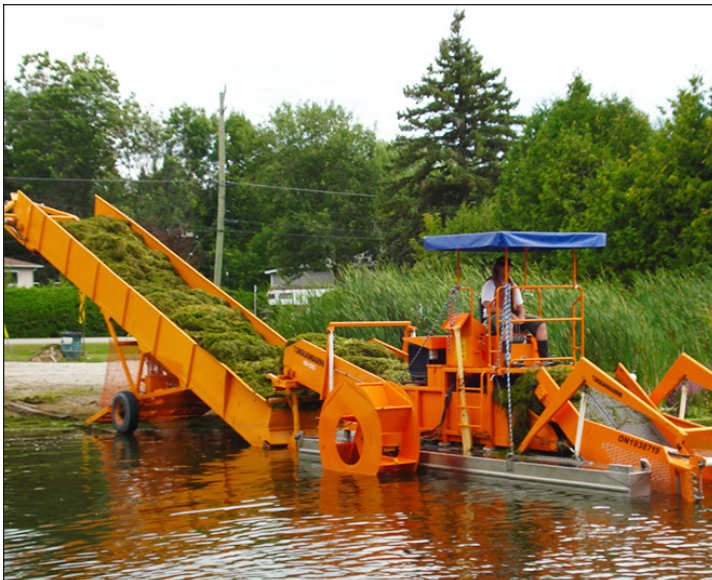
Using a power barge makes weed collection very efficient
